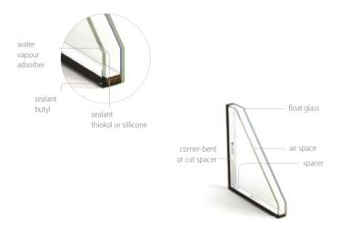
First modern tight IGUs were developed in 1950s, but they started to be produced and used commonly in buildings about 20 years later. The technology owes its development to the deficit in generation of thermal energy to heat buildings.
